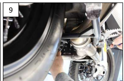
6 Prepare step (7) with Tbhc 8x50mm + 2 M8 Washers + 1 Em8f
