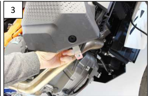
2 Place the clamped bolts as shown (2) and fix it on the bike on left and right sides using the OEM screws + M6 Washers + Em6f (3)
